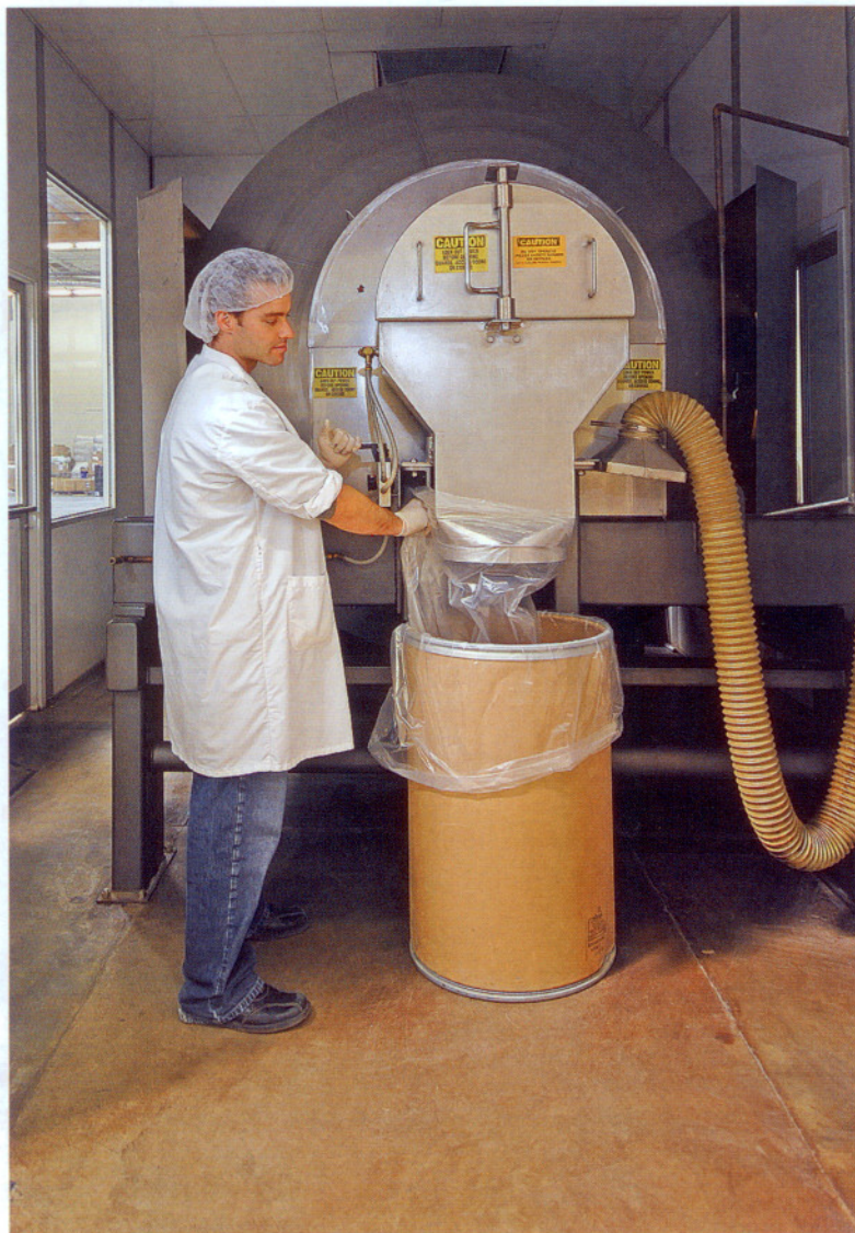
Internal mixing flights elevate the material which is discharged through a plug gate valve into plastic-lined drums.
